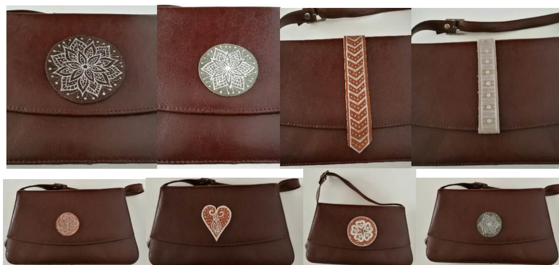
Fig.7: Different ornamental elements with silver foil and silver ion based paint applied on purses
